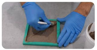
**Step Four**Brush 1-2mm facing coat into your mould.
