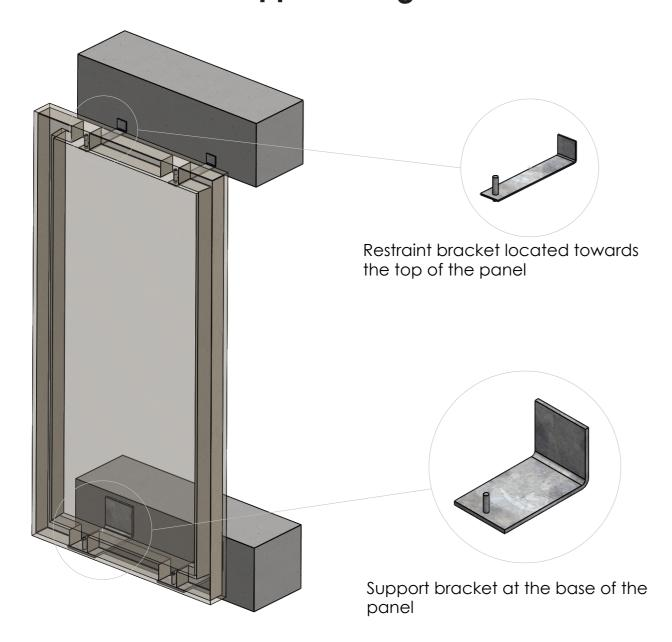
Panel spans between fixing points.
