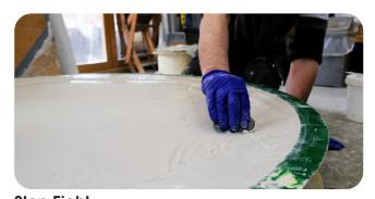
**Step Eight**Finally, pour sufficient product into your mould to meet your desired level. Leave, then demould.
