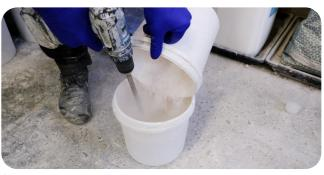
**Step Two**Weigh and mix your base and liquid to ratio.
